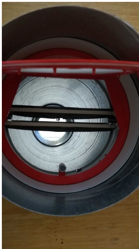
Photo C. 1: Installation of the specimens (SC60-COSMO)
